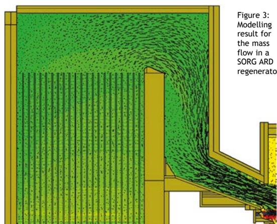
Figure 3: Modelling result for the mass flow in a SORG ARD regenerator.
