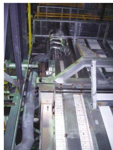
Figure 4: SORG ARD regenerator on an end-fired furnace.
