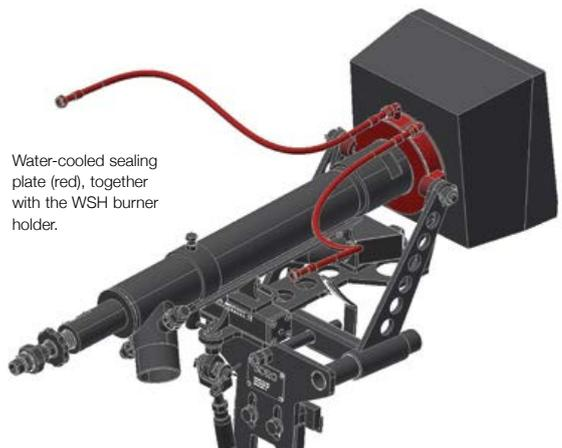
Water-cooled sealing plate (red), together with the WSH burner holder.
