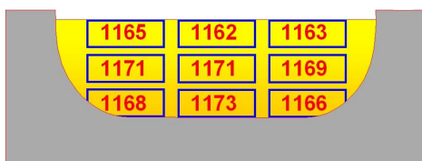
Figure 8 – temperature distribution with favourable tolerances : THI = 97,4
